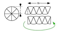
Area of Parallelogram = Base × Height  $Area = \frac{1}{2}(2\pi r) \times r$   $Area = \pi r^{2}$
