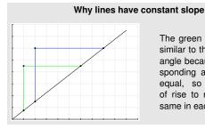
The green triangle is similar to the blue triangle because corresponding angles are equal, so the ratio of rise to run is the same in each.
